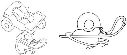
3. With the vehicle in park, put the strapping system around your tire. The strapping system should be centered over the tire.
