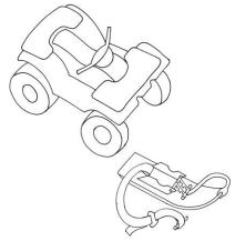
2. Drive vehicle's front passenger tire into the saddle until the tire pushed up against the front cross plate. DO NOT put vehicle in 4WD during operation.
