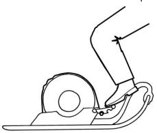
5. With the cam pin inserted in the cam lever, push the cam lever down with your foot on the cam lever arm. **CAUTION**: Do not place fingers on or around the cam lever or around the pinch point by the cam lever. Fingers can be pinched.
